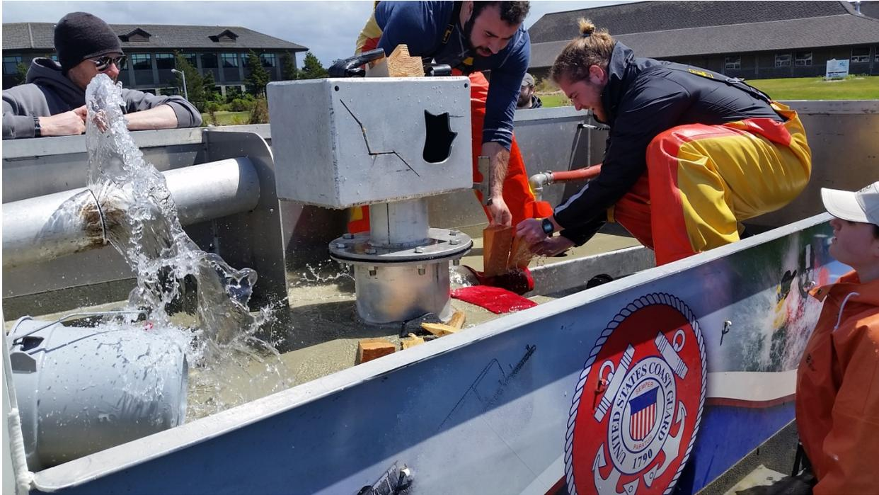
**Figure 13 - Trainee teamwork plugging leaks on the USCG DC trainer at Newport**
